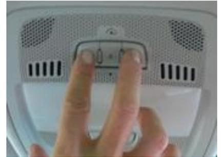
2. Press the appropriate HomeLink button I, II or III which you want to program and keep holding it until the diode starts flashing slowly.
