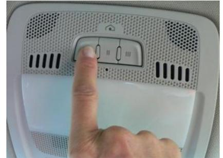
In the case of a standard code, the HomeLink diode is constantly illuminated throughout the transmission process. For use with compatible systems, no further action is necessary.
