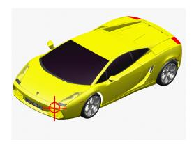
The corresponding HomeLink transmitter is located at the front left<sup>1)</sup> in the bumper, under the headlamp.
