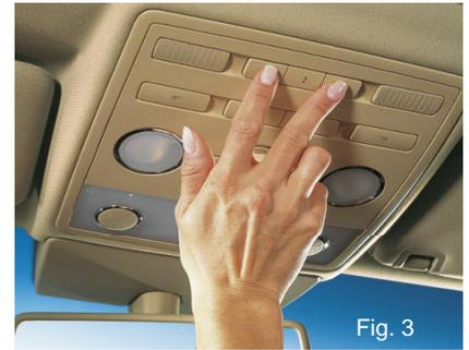
2. Hold the original remote control of the device you wish to train at a distance of 5-30 cm away from the HomeLink transmitter unit, keeping the background light behind the HomeLink buttons in view all the time.
