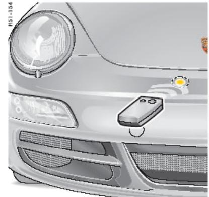
4. The fog lights blink **three times** to indicate that programming has been successful.
