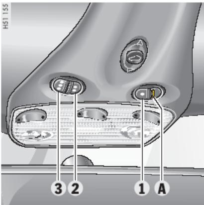
The HomeLink control panel with buttons 1, 2 and 3 in the roof area, immediately behind the interior light. Light diode A to display status.
