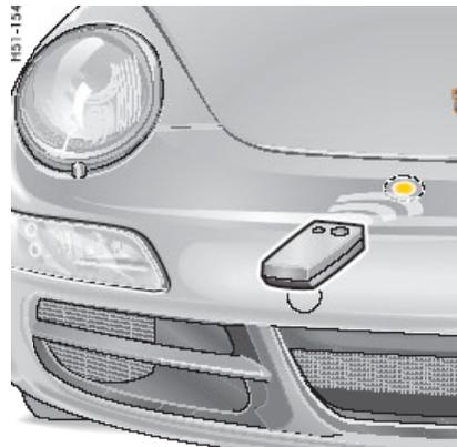
The HomeLink transmitter unit in the front bumper, about 10 cm to the right<sup>1)</sup> of the vehicle's centre.
